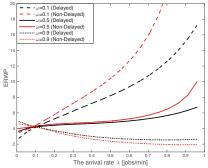
Figure 5: Comparison of ERWP values for the offloading models under different arrival rates
